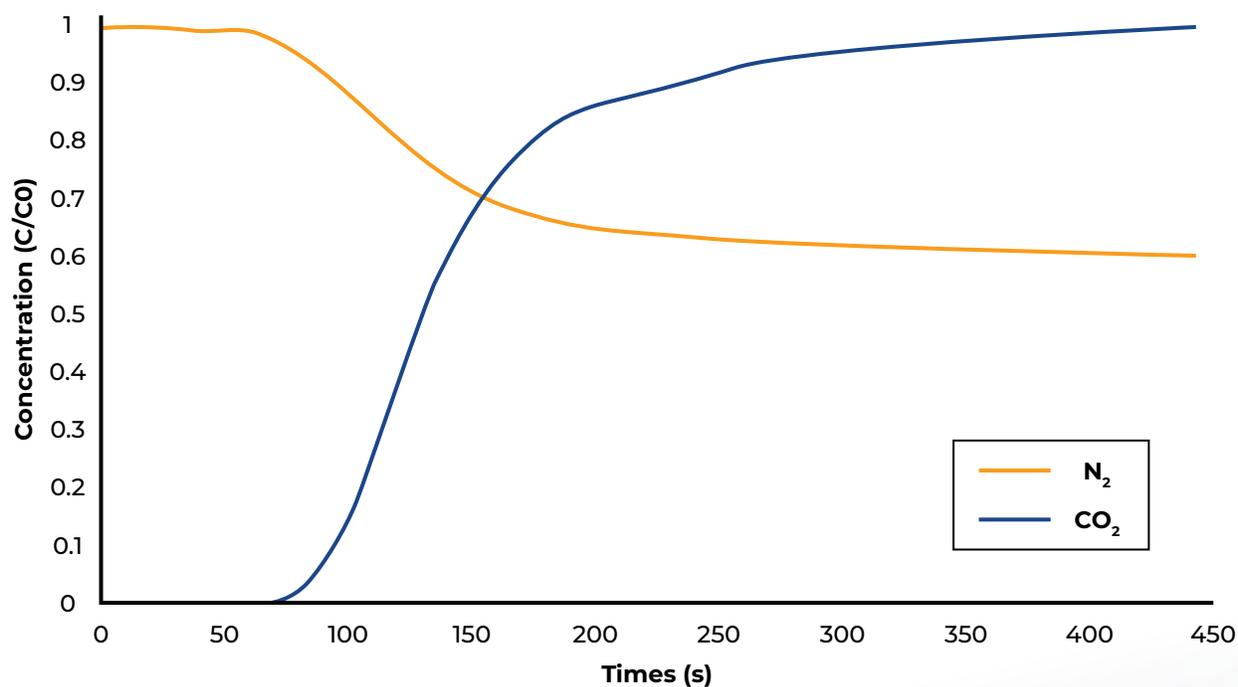
Figure 2. CO<sub>2</sub> breakthrough adsorption in zeolite 13X.
