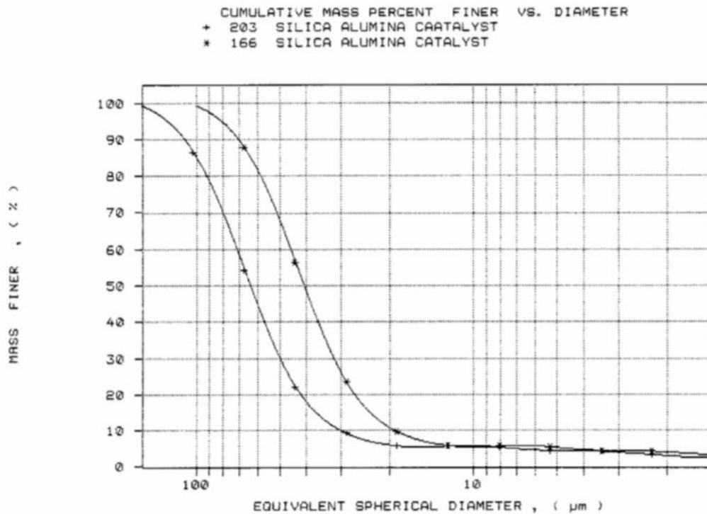
Figure 2. SediGraph PSD for Si/Al catalyst powder using (+) a sedimentation density of 1.65 g/cm<sup>3</sup> and (\*) using a sedimentation density of 2.60 g/cm<sup>3</sup>.
