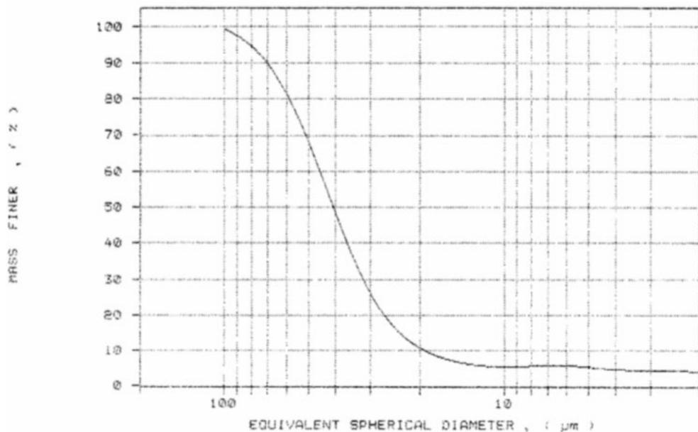
Figure 1. SediGraph PSD for Si/Al catalyst powder using a skeletal density of 2.60 g/cm<sup>3</sup>.
