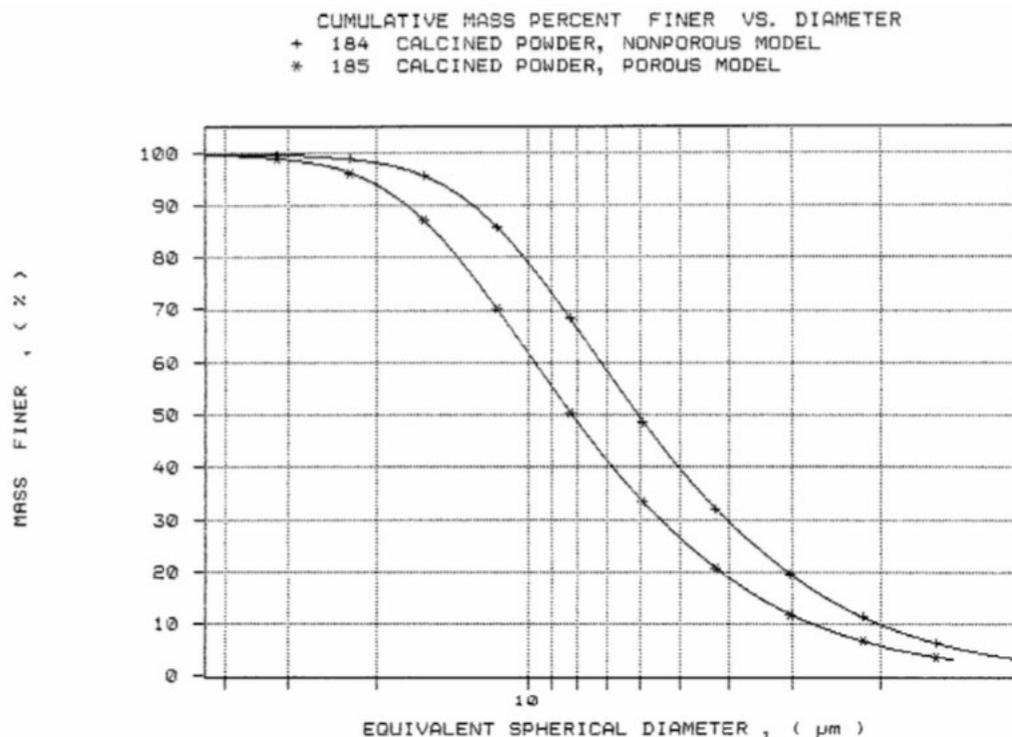
Figure 3. The SediGraph PSDs for the calcined product using (\*) a density of 2.05 g/cm<sup>3</sup> and (+) a density of 2.92 g/cm<sup>3</sup>.
