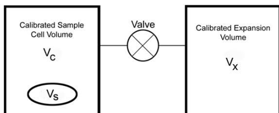
Sample volume is determined from the known cell and expansion volumes and from measured pressures.
