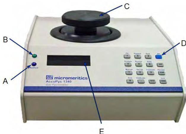
The sample chamber, located on the top panel, is where the sample cup is placed for analysis.
