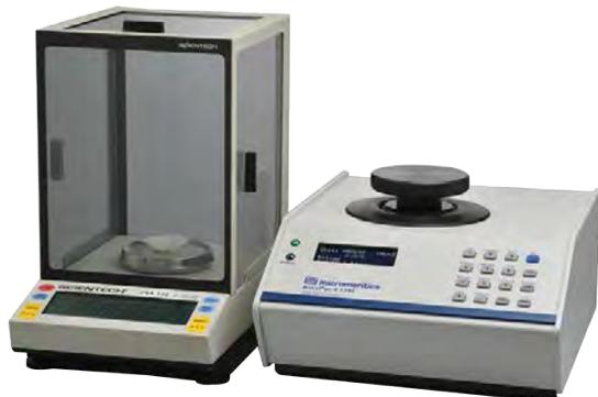
An analytical balance can be connected to a serial port on the computer and used to transfer the sample's mass directly to the AccuPyc II application.
