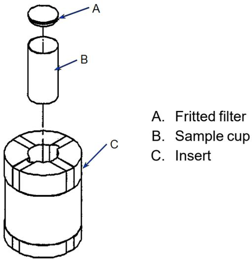
The inserts for the 2000 cm<sup>3</sup> systems are installed and removed with a special tool.
