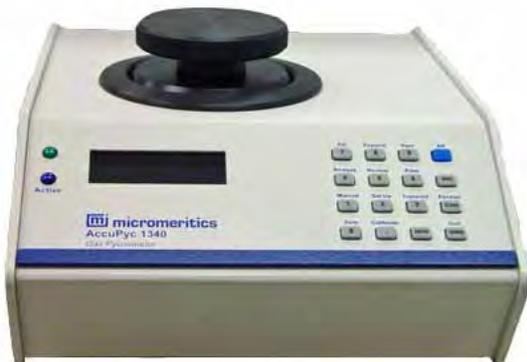
Gas pycnometry is recognized as one of the most reliable techniques for obtaining true, absolute, skeletal, and apparent volume and density. This technique is non-destructive as it uses the gas displacement method to measure volume. Inert gases, such as helium or nitrogen, are used as the displacement medium. Density calculations using the gas displacement method are much more accurate and reproducible than the traditional Archimedes water displacement method.
