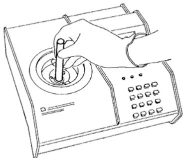
5. If using a fritted filter cap, place it onto the top of the insert.
