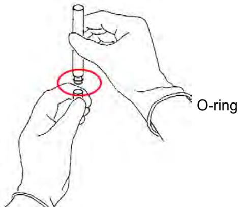
4. Place the cup into the insert, then tilt the tool to one side and remove it from the sample cup.
