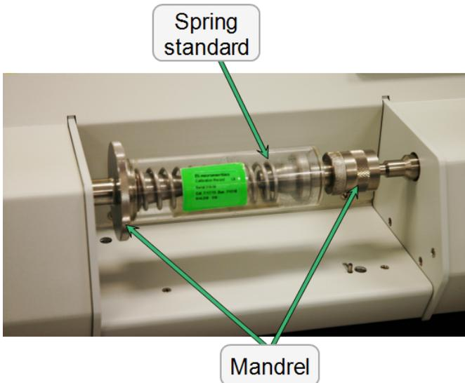
1. Attach the base of the force calibration tool to the face plate (left side threaded mandrel). Tighten firmly
