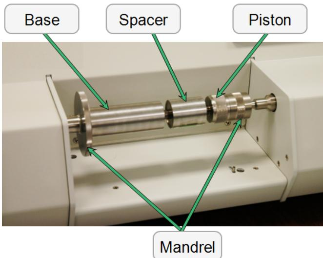
1. If using a spacer, insert the spacer onto the piston, otherwise skip this step.
