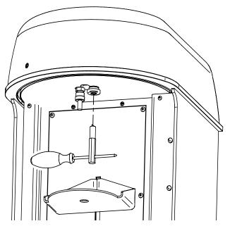
5. Repeat steps 1 through 4 for the balance port, using the  $2-\mu m$  frit.
