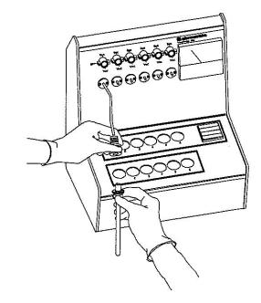
c. Attach the sample tube to the connector on the vacuum tube by turning the vacuum tube connector nut clockwise to tighten.
