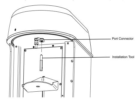
4. Using a 1/2-in. wrench or screwdriver, tighten the installation tool, hand-tight plus 1/4 turn.
