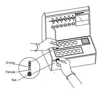
b. Attach the 1/2-in. O-ring and 1/2-in. ferrule that are included in the VacPrep kit to the connector and tighten the connector nut.
