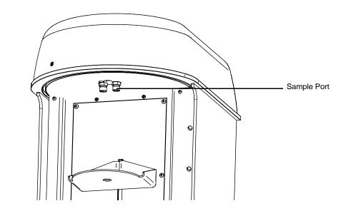
2. Assemble the 40-µm frit, O-ring, and connector included in the kit. Install them in the sample port connector as shown below.
